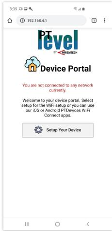
Once you are connected to the PTLevel WiFi, open your device browser and type **192.168.4.1** into the address bar.
