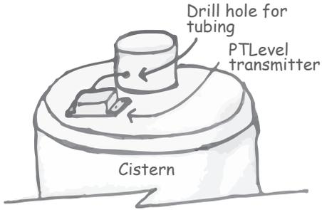
The main idea is to mount the device outside of the tank.
